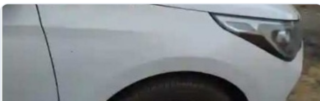
Fender RHS: Repainted Clearcoat
